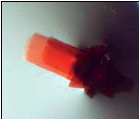
Figure 4.7 Cytochrome c nitrite reductase crystals. Crystals of NrfA were formed using the vapor diffusion method. NrfA ( 1 \mu\text{l} ) at a concentration of 10 \text{ mg ml}^{-1} was mixed with 1 \mu\text{l} mother liquor containing 100 \text{ mM} HEPES, pH 7.5, 20% PEG 10K and incubated in hanging drop trays with a 1-ml well solution at 4^\circ . Crystals typically developed in 5–14 days.
